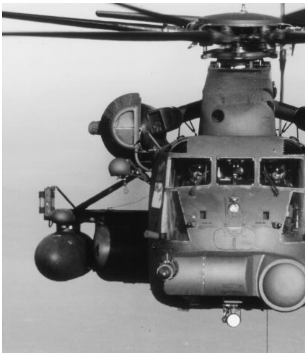
A front close-up view of an MH-53J helicopter of the 21st Special Operations Squadron, equipped with the Pave Low infrared system for night operations, in flight near the English coast.
