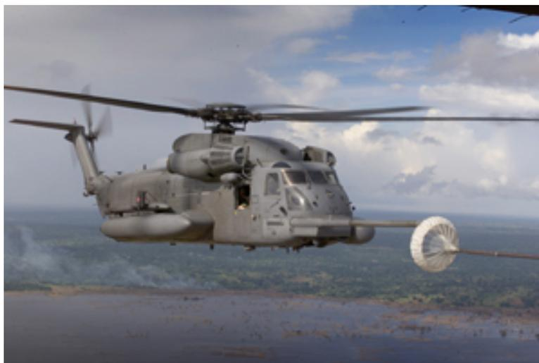
**Ability of PAVE LOW to refuel in midair can make the SAR difference.**
